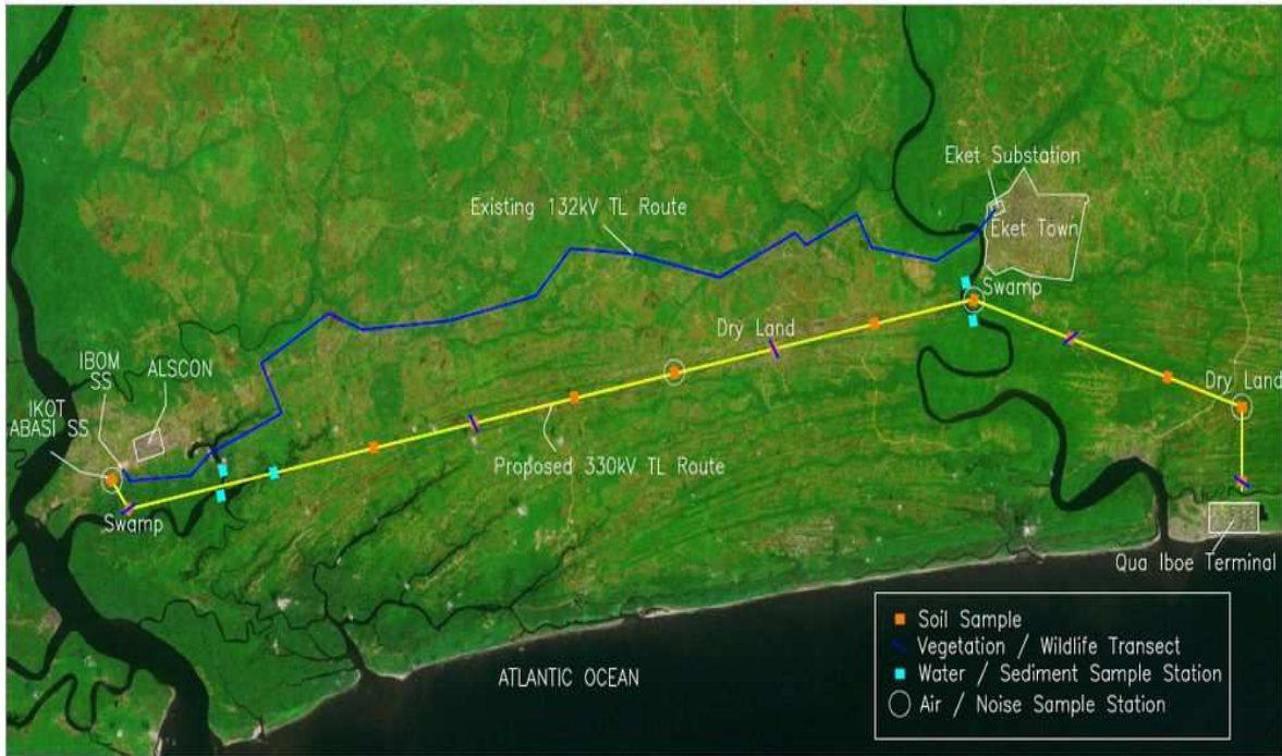
Figure 2: Locations of environmental baseline study sampling stations relative to routes proposed for QIT to Ikot Abasi Transmission Line Project.
