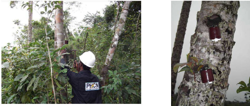
Figure 1.8: Installation of Ogawa Passive Samplers
