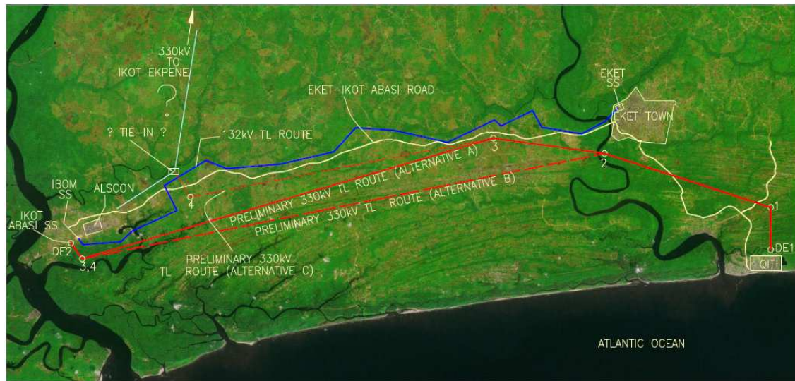
Figure 2.2: Existing 132 kV T - line Eket to Ibom (blue), Recommended 330 kV T-line QIT – Ikot Abasi SS Alternatives (red)
