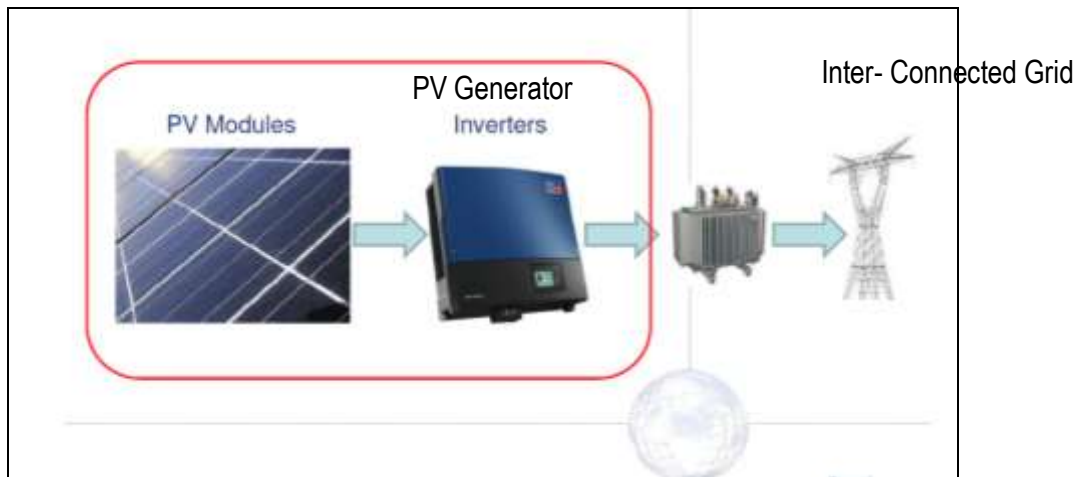
Figure 4: Components of a Grid Connected PV System
