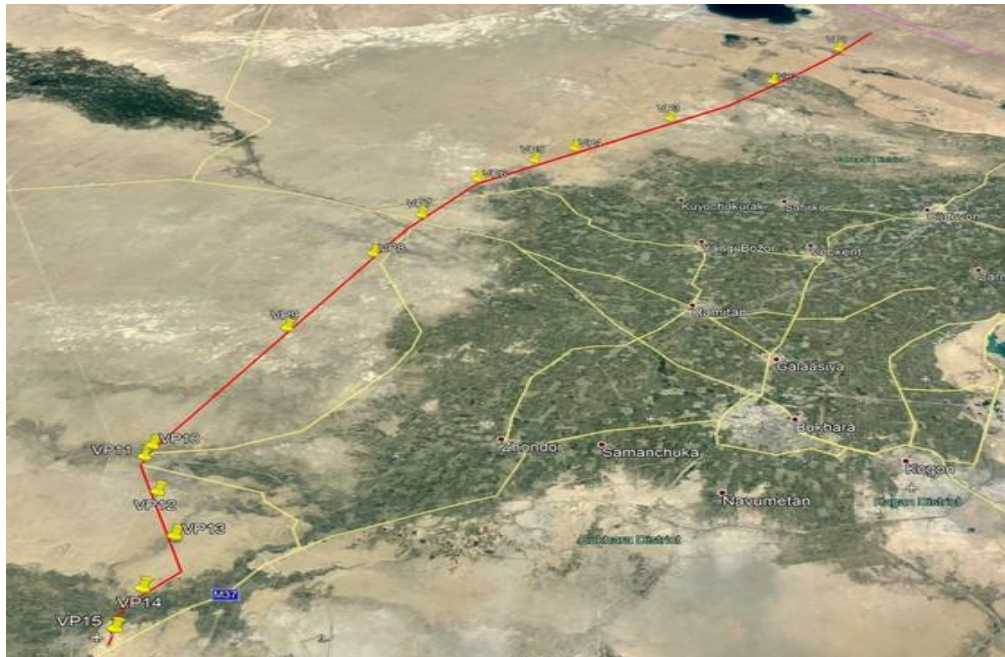
Figure 2-66 Survey points on the Bash-Karakul OHTL Route
