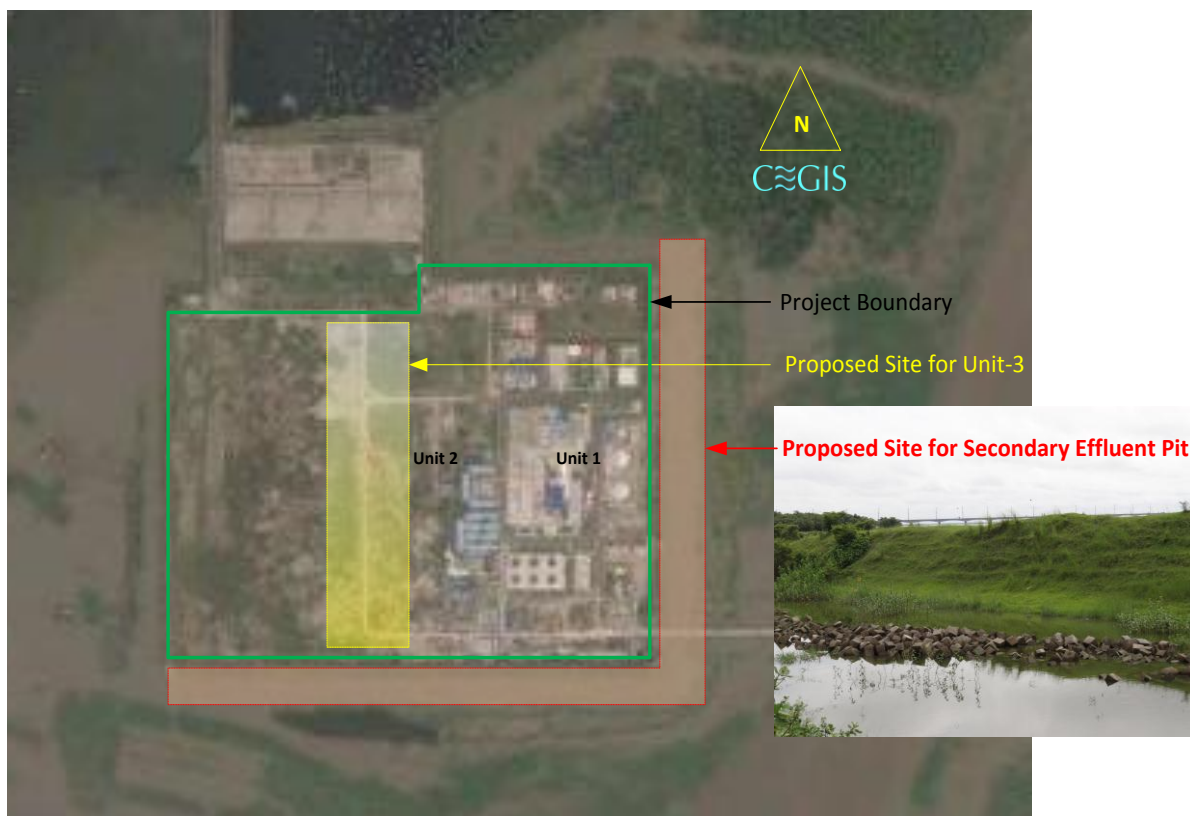
Figure 8-3: Proposed layout for creating secondary effluent pit
